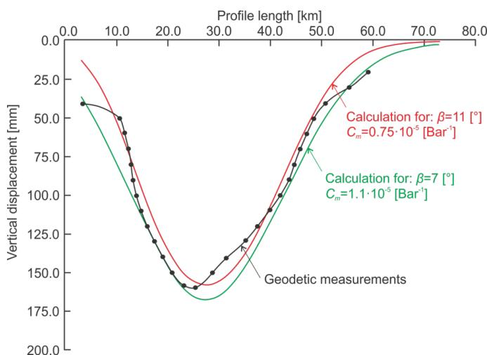
Fig. 7. Comparison of the measured and theoretically calculated subsidence basin for the Groningen gas field (as of 1987) (Sroka et al. 2018a)
