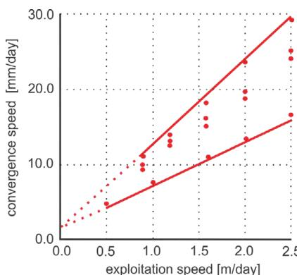
Fig. 3. Relationship between convergence velocity and advancement velocity of the mining front
