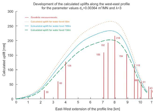
Fig. 8. The uplift development along the east-west profile for a sample coal mine (Preusse and Sroka 2015)
